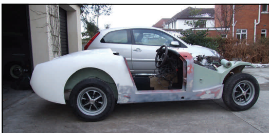
Above left: PO1 1028 as purchased for project. Above right: The Midget has lost most of its bodywork and any exposed corrosion was cut out and new metal MIG welded in. Left: The restored tub was cleaned and treated with specialist paint prior to fitting the new Frogeye bodyshell.
